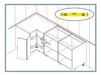
12. Set the next cabinet tight to the first cabinet and use clamps to hold it in place while you level it and make sure that the front edges are flush. Attach the two cabinets together using 1 1/8" particle board screws. Attach the cabinet to the wall with 2 1/2" screws into the studs. Continue with the same process for all base cabinets.
