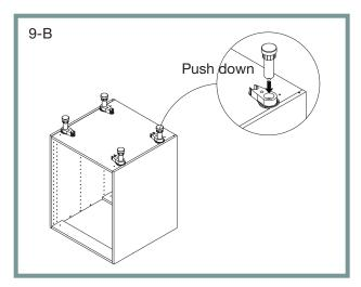
9a/9b. When installing the adjustable legs, start by inserting the leg portion into the factory installed base. Use strong pressure to push the leg into the base, and then adjust to the desired height. This should be 4 1/2" for normal use.
