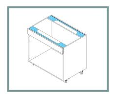
When installing a sink or cooktop, trimming the top support rails may be necessary. Using the template supplied by the sink or cooktop manufacturer, cut the top rails as required using a jigsaw.
