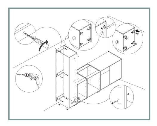
13. When installing tall cabinets, make sure they are level and plumb. Attach to studs, using 2 1/2" screws into all studs at the top, middle and bottom, screwing through the hanging rails. If the tall cabinet is against other cabinets, use your clamps to hold it in place and screw the cabinets together using 1 1/8" screws.
