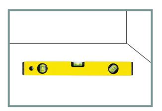
2. Before beginning installation, you must first find the highest point of your floor by checking it with a level.
