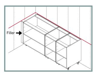
11. For designs without a corner cabinet, start with the first cabinet leaving space for a filler, as per your plan.
