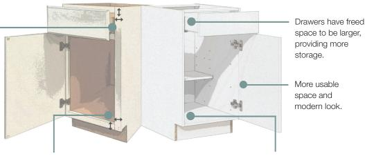
Frame creates smaller cabinet opening, obstructing access, plus frame edge can snag storage items.
